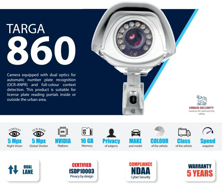
**Dual lens** camera (OCR and context) for automatic reading of number plates and dangerous goods (Kemler), **dual lane**, equipped with a 5 Mpx Global Shutter OCR sensor, with 12-40mm varifocal lens (3x zoom) and a 5 Mpx Sony Night Vision high-sensitivity colour context sensor with 12 mm fixed lens.
