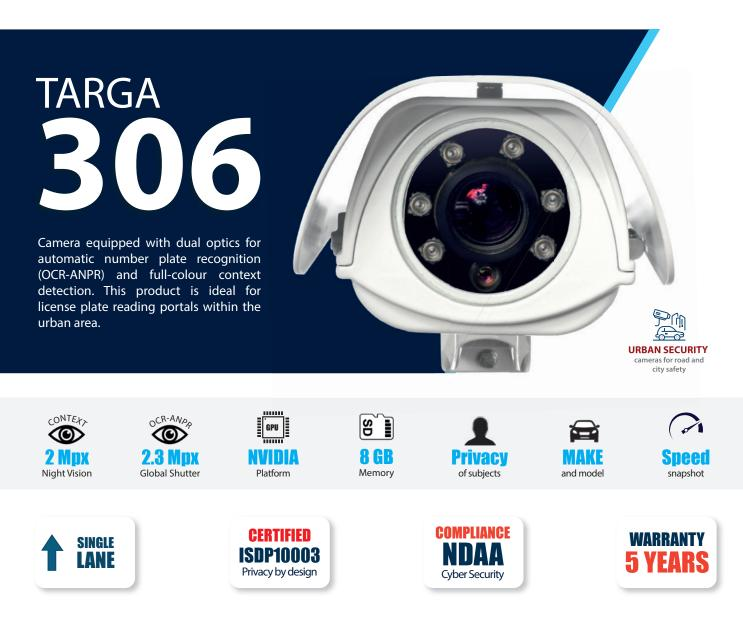
**Dual lens** camera (OCR and context) for automatic reading of number plates and dangerous goods (Kemler), **single lane**, equipped with a 2.3 Mpx Global Shutter OCR sensor with a 25 mm fixed focal lens and a 2 Mpx Sony Night Vision high-sensitivity colour context sensor with a 12 mm fixed lens.
