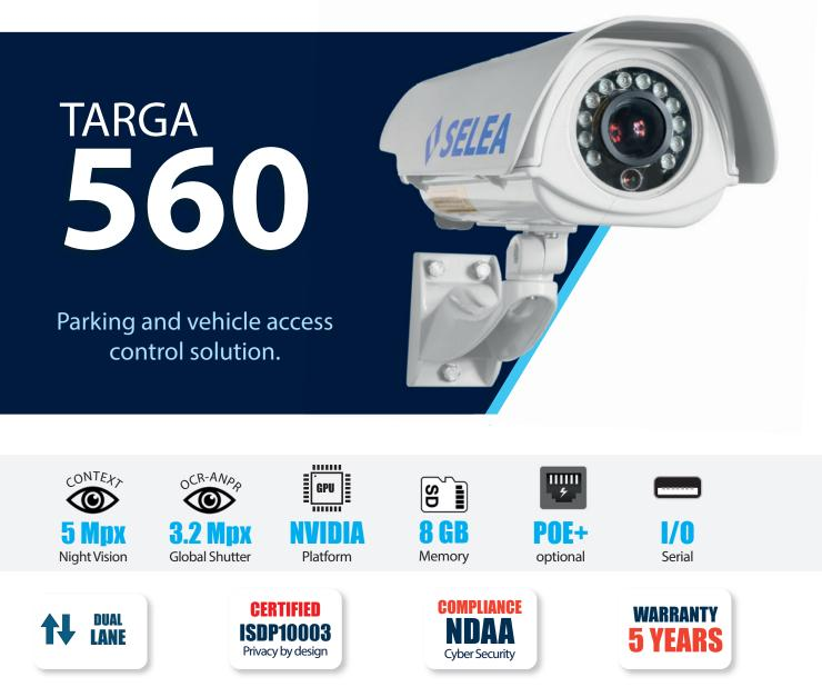
ANPR camera for parking and access control systems, for OCR recognition of number plates and dangerous goods (Kemler), with **high accuracy** even in critical conditions such as dirty and deteriorated number plates, during the day and night. License plate reading solution for those who want to create a professional access control system also for the control of heavy vehicles on widened gates (7 m).
