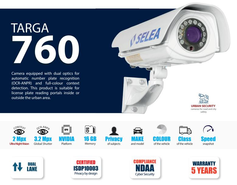
**Dual lens** (OCR and context) camera for automatic reading of number plates and dangerous goods (Kemler), **dual lane**, equipped with a 3.2 Mpx Global Shutter OCR sensor, with 12-40mm varifocal lens (3x zoom) and a 2 Mpx Sony Ultra Night Vision high-sensitivity colour context sensor with 12 mm fixed lens.
